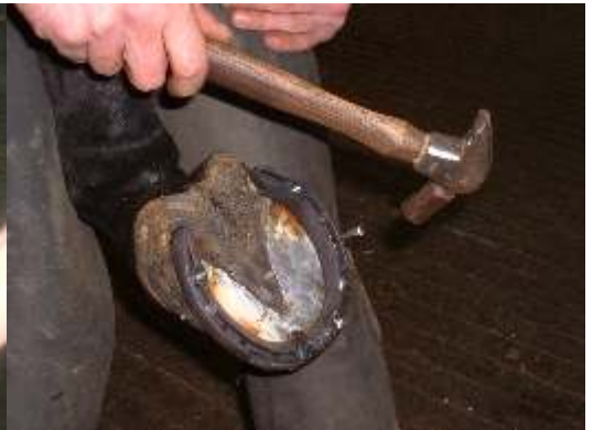
Nailing the hot shoe to the foot
